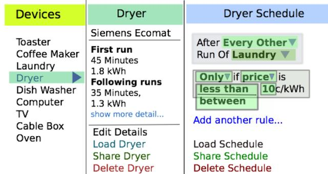
**Figure 5: Sketch of EDC<sub>E-SIM</sub> Interface for Scheduling Appliances**
