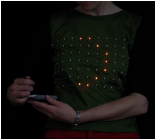
Figure 3. A programmable tanktop shirt. Here, the wearer is "reprogramming" the shirt wirelessly with a new starting cellular automaton pattern.
