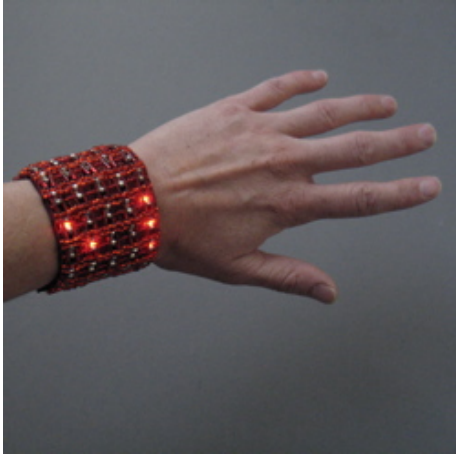
Figure 2. A programmable bracelet with an array of LED sequins as a display.
