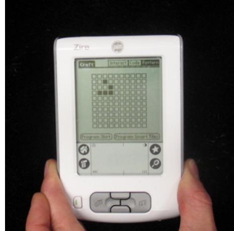
Figure 4. A close-up of the handheld PDA interface for reprogramming the tanktop shirt in Figure 3.
