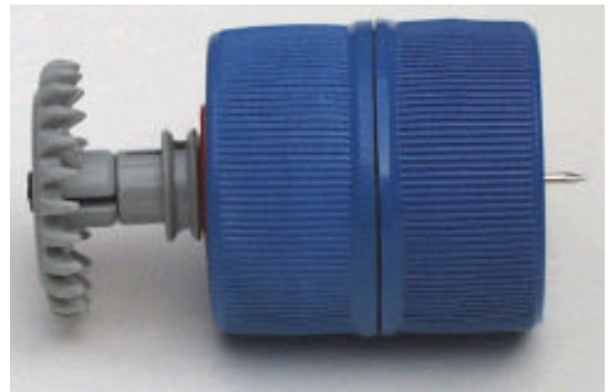
Figure 4. A side view of an early rototack. The "pin" may be seen at right; the rotating head at left. The power source and internal computer is hidden within the casing at center.
