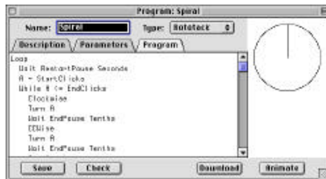
Figure 5. A mockup screen of a rototack programming environment. As envisioned here, the program is written and edited in the text window at left; by pressing the Animate button at bottom right, the program will be interpreted and, while it runs, the graphical schematic of the tack will show the rotation that a physical tack would exhibit. Once the user is satisfied with the behavior of the program, he can download it to an actual tack.
