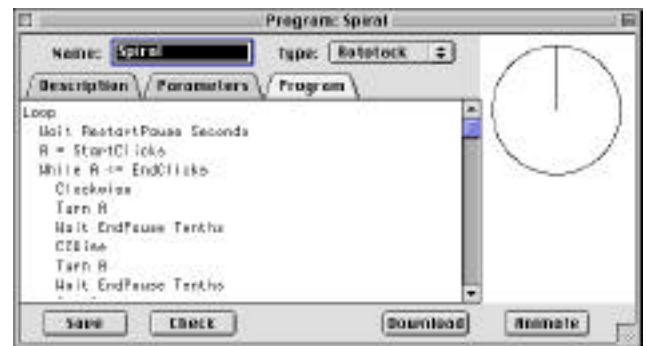
Figure 5. A mockup screen view of the tack programming environment described in the text. The frame at left shows the text of the program in construction (views of the program’s parameters, and a textual description of the program are also available in this frame). At right, an abstract representation of the tack (as seen from the top). The Animate button toward the bottom right links the running program to the graphical tack.
