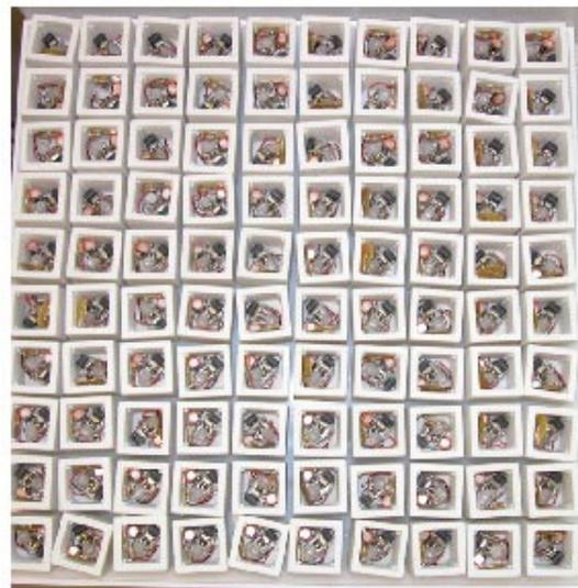
**Figure 12. A ten-by-ten array of "opened" smart tiles illustrating the construction of the individual pieces.**
