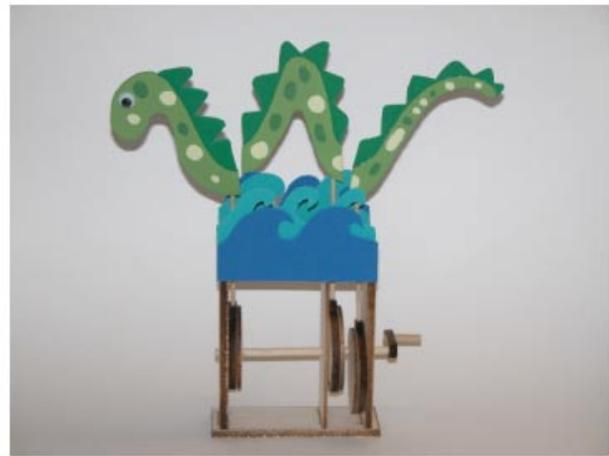
**Figure 4. A mechanical sea monster automaton; the foam core monster, cams, and box structure were printed on a laser cutter.**
