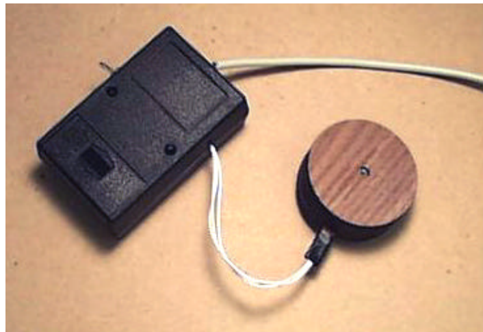
Figure 2. The Rototack connected to its interface port for downloading a newly-written program. At right, out of the photograph, is a desktop computer
