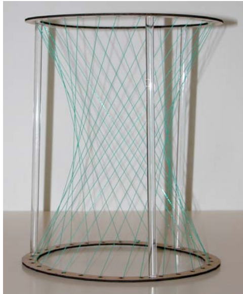
Figure 6. A string hyperboloid produced by weaving string between two parallel ring frames. The rings are separated and supported by three clear acrylic dowels.
