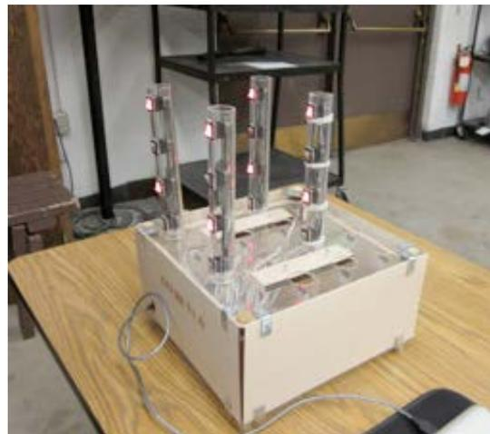
Figure 1. The *UCube* system, shown here with four of a possible 16 towers in place, with two lighted switches on each tower, together indicating the 8 vertices of a cube "2 units" in size.
