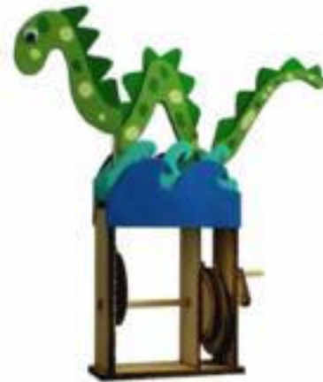
Figure 6. (top) A set of mechanical elements printed out in wood. The element at the left of this set—an eccentric cam with a ring follower—is used several times over in the construction of the homemade sea monster automaton at the bottom of the figure.
