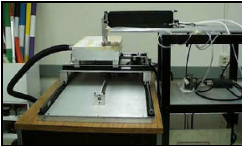
Figure 5. A laser cutter in operation. Here, the table is moving underneath a (stationary) laser to produce wooden cutout pieces, much like those shown in Figure 4.
