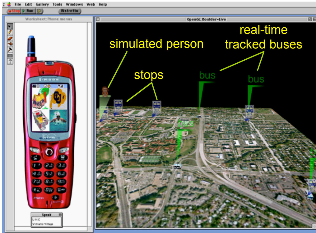
Figure 5: Agent-based prototype showing a mobile prompting device synchronized with display of real-time bus system.
