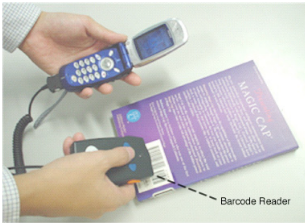
Figure 8: Hardware configuration for the smartphone-based implementation
