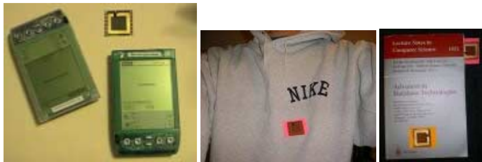
A Prototype of QueryLens uses a database server, PDAs and RFID tags. RFID tags are so small that they can be attached to or embedded in many different kinds of physical entities.
