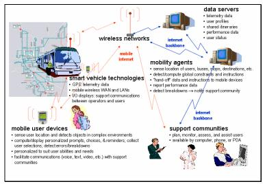
Figure 1: A proposed architecture to support mobile users and their support communities
